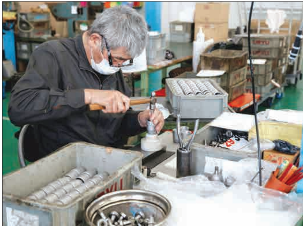
A worker assembles an air drill at the factory of manufacturer Katsui Kogyo in Higashiosaka.
